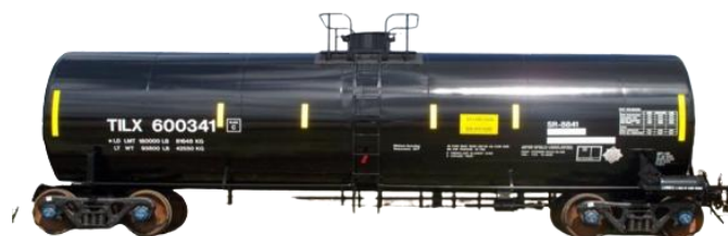
Above: A liquid chlorine rail car, equipped with additional protections meant to reduce the risk of an accidental release, like reinforced walls and rollover protection
