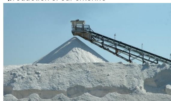
Below: Looking at our salt storage on site. We barge in solar-dried ocean salt from the Baja region of Mexico for the production of our chlorine
